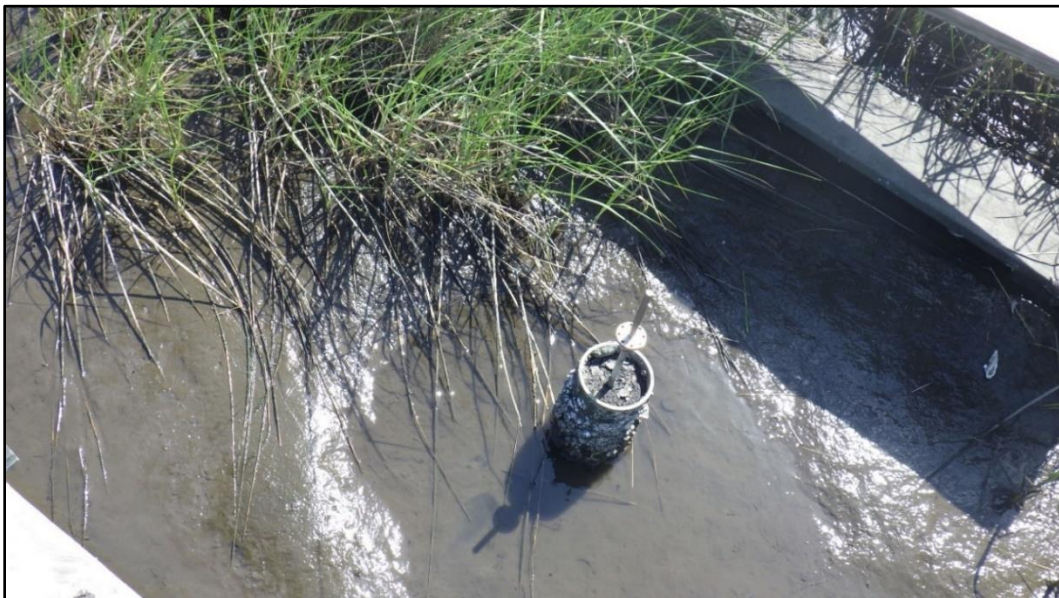
Figure 66. CRMS0258 RSET station in the fall of 2025, 13 years after the top 30 cm of soil was removed containing mostly shallow open water, mudflats, and minimal vegetation
